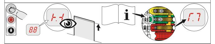
3. Move to close position 5cm above the ground and adjust S5 pre-limit switch
