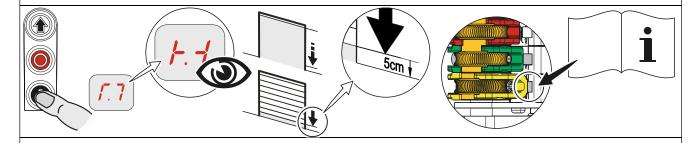
4. Move to close final limit position and adjust S4 CLOSE limit switch
